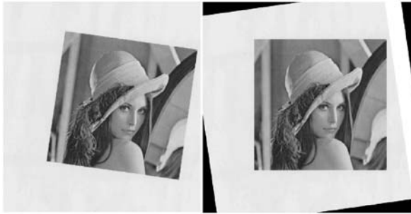
Fig. 5. a) Watermarked image after print-scan process. b) Watermarked image after correction of rotation and scale.
