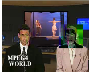
Fig. 12. Conditional Access control with different access rights of 2 ROIs; ROI 0 (QCIF, 15fps, base quality), ROI 1(No access right)
