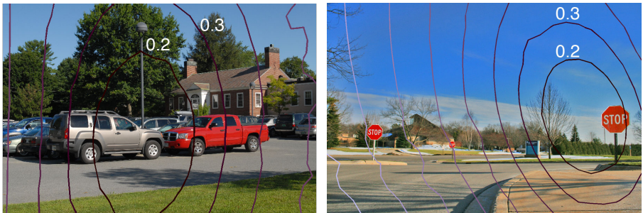
Fig. 9. Shown in each panel are authentic images with superimposed level curves showing the deviation of the estimated principal point from the true principal point as a function of spatial position in the image. The principal point for the left image was determined from the left-most car’s wheels, and for the right image, the known geometry of the stop sign.
